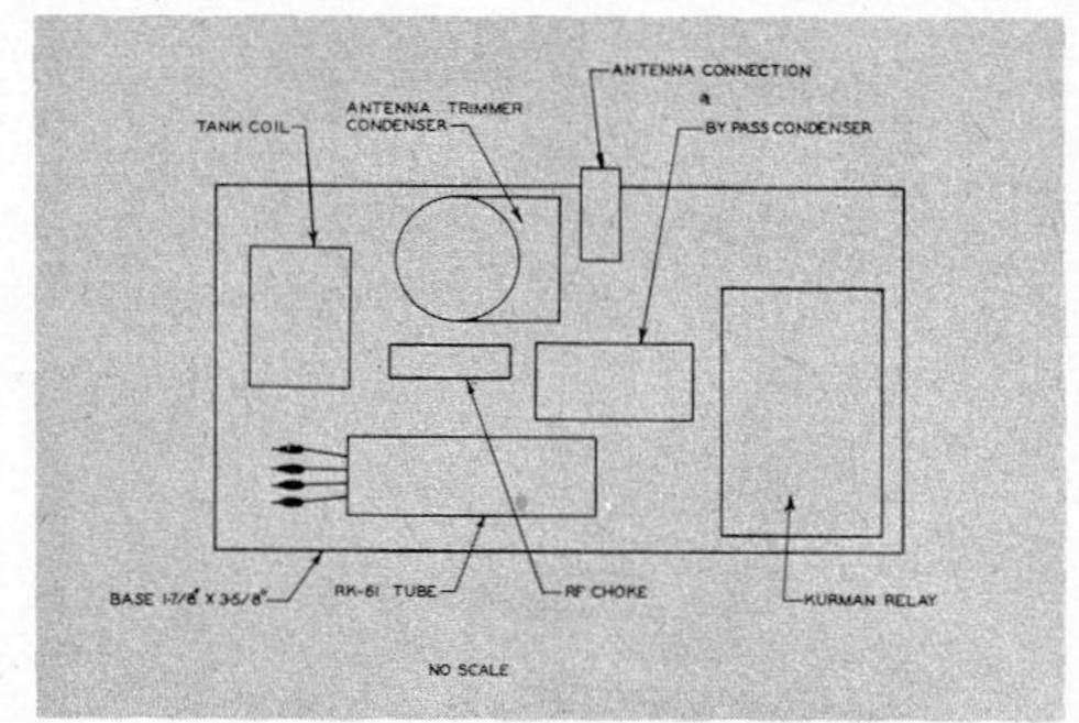
In the receiver, left, above, the author has remounted all the parts on one side of the base to facilitate the sponge-rubber mounting described. Above, right—diagram identifies all parts in the picture. The tank coil is cement covered before tuning up so that receiver frequency remains stable.
