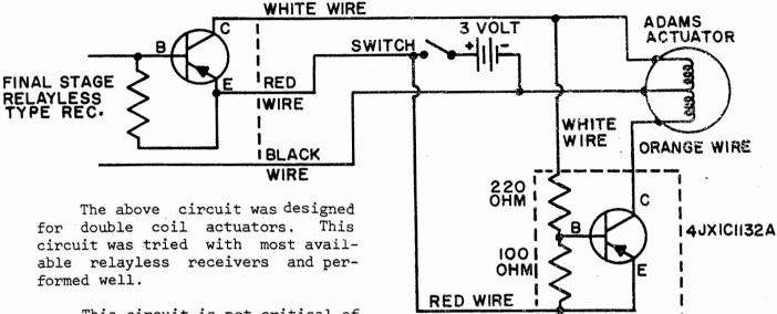
This circuit is not critical of selection of transistors, since the 2N3638, 2N1303, T1046, and the 4JX1Cl132A were tried and all performed well. The circuit is very tolerant of resistance values used.
