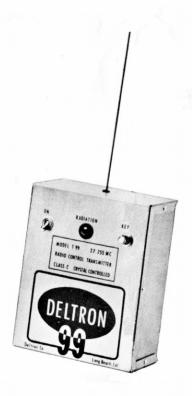
The T99 is a lightweight, sturdy, long-range R/C transmitter, crystal controlled for operation on the citizens frequency of 27.255 MC. Built around a newly developed printed circuit that assures high radiation and uniformity of output, it will give years of superior performance if it is not abused.
