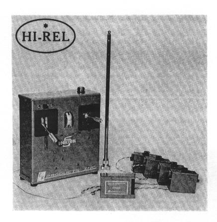
IN ADDITION TO ITEMS SHOWN ABOVE COMPLETE MS-2-5 SYSTEM INCLUDES BUILT-IN CHARGERS. SWITCHING HARNESS, A.C. AND D.C. CHARGING CORDS, AND NICKEL CADMIUM BATTERIES.
