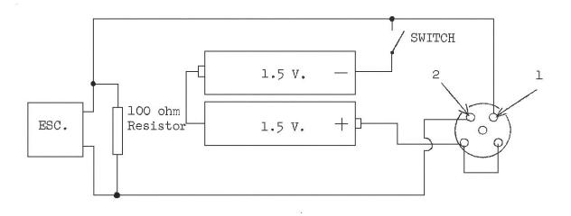
INSTALLATION USING TWO SETS OF BATTERIES:
