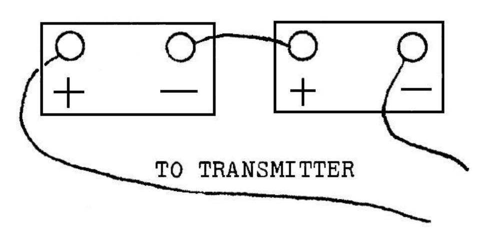
OBSERVE POLARITY ON 12 VOLT BATTERY. RED LEAD GOES TO POSITIVE SIDE OF BATTERY.
