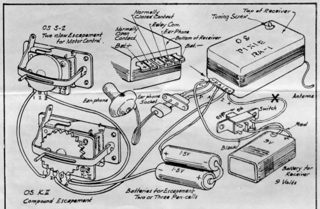
Remarks: X mark is to show the place for inserting a meter when you need to test.
