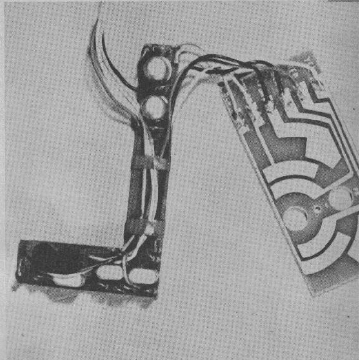
Completed and wired, ready for installation in the servo can, your transistorized assembly should look like this. Photograph is exact size.
