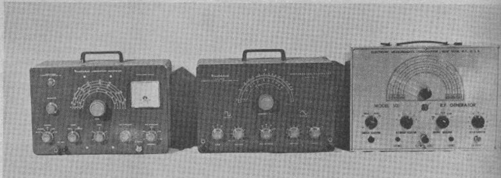
Signal generators, both RF and audio types, in serious fan's laboratory. Used with VTVM or 'scope. The most versatile test instrument available to the R/C fan is the Volt Ohm-Milliammeter—VOM.
