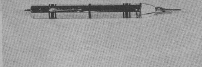
Home-made signal injector in penlight case for troubleshooting.
