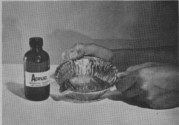
4. After the PC board is exposed it is placed in a metal or glass (not plastic) dish and covered with developing solution. Gentle rocking for one minute removes all the unwanted photo resist leaving only the exposed circuit covered. Air drying without blowing or touching for 30 seconds makes the board light-safe.
