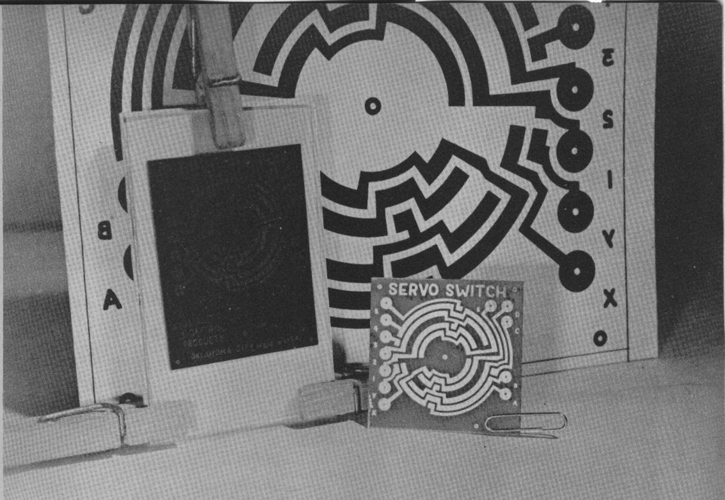
Any circuit that can be drawn on paper—usually two to four times up—however complicated, easily can be transferred to copperclad board.
