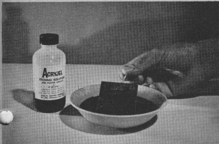
5. The developed PC board is placed in a plastic or glass (not metal) dish and covered with etching solution. Pre-warming the solution in a hot water bath and frequent agitation greatly speeds the process of removing all unwanted copper.
