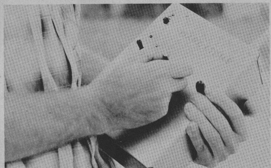
Transmitter is cradled in hand with heel of hand resting on case. Thumb, forefinger for stick.
