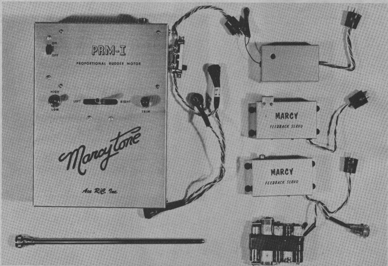
Complete system, X-mitter left and, right, top to bottom, receiver, engine and rudder servos and battery pack. Wiring harness includes switches.
