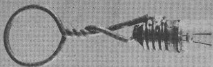
The tune-up loop with pilot lamp. Loop is #20 wire, the ends soldered to #48 pink bead lamp.
