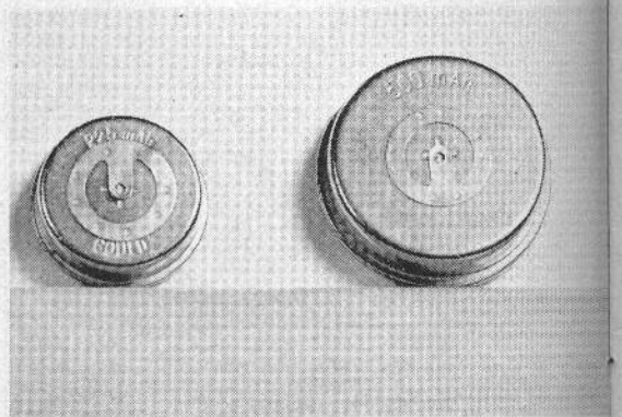
Some representative cell types. Recommended charge and discharge rates should never be exceeded because of faster disintegration of the electrodes. Popular button-cell sizes shown are 225 and 500 mah capacity. Voltage is 1.2.
