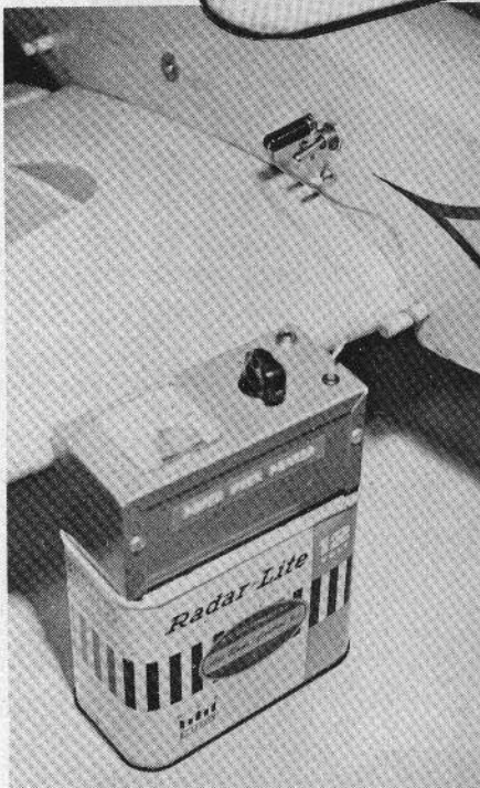
Above—Peaker mounted on 12V Burgess lantern battery (Type TW-2). Lafayette meter 0-50 or 0-100 ma, and Bud Minibox. At left, peaker shown plugged into plane. Drawing, below, shows how the device is assembled. Unit costs less than $10 when home-built.
