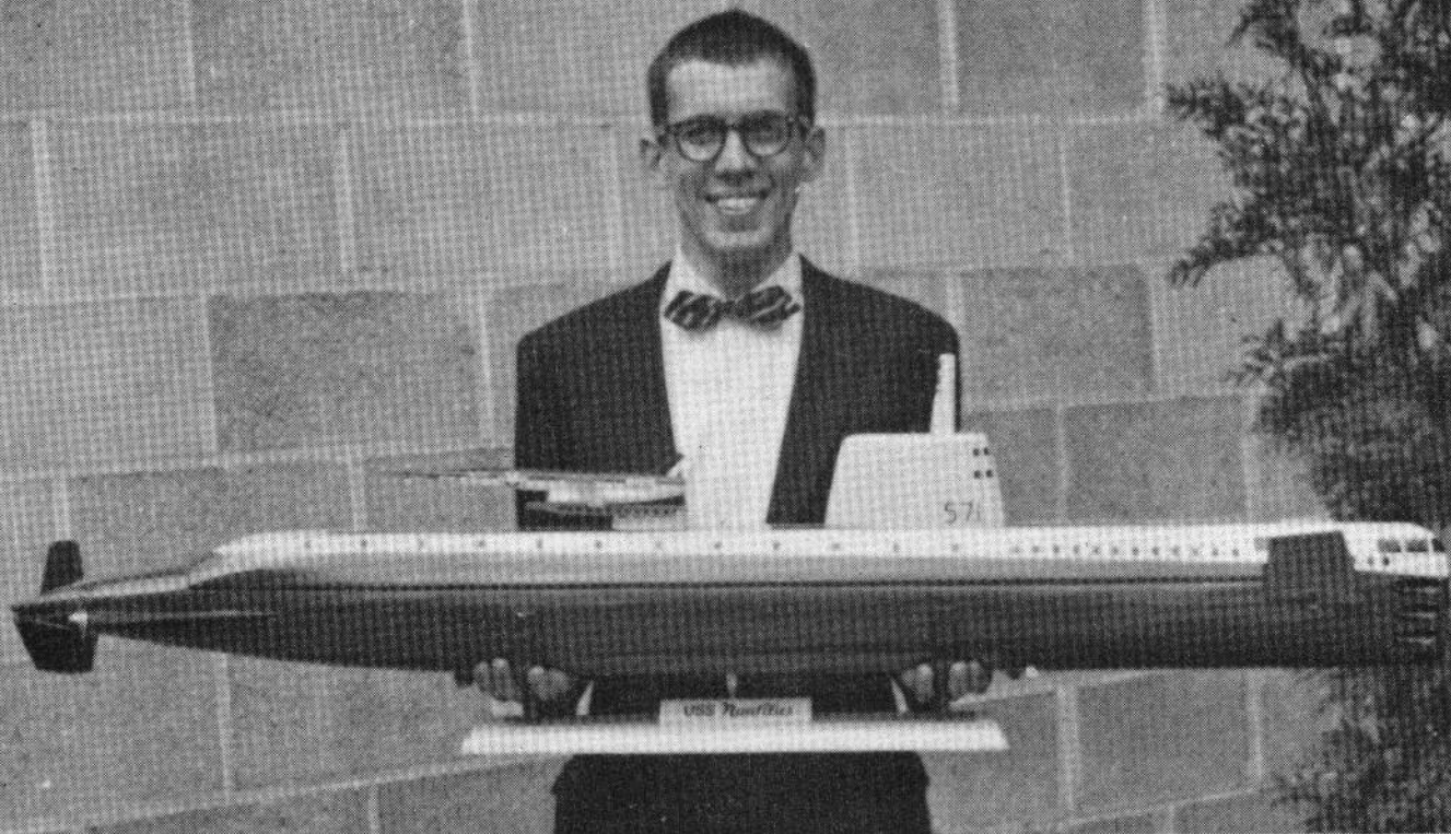
The author and the 56-in. model. It has a beam of 5¼ in., weighs 31 lbs. Hull is constructed from white-pine laminations.
