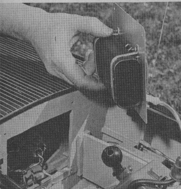
Tank made from half-pint can—hence the boat name—clamped to a hatch which closes radio compartment under foredeck. Visual fuel-level gauge and quick-fill caps. Servos placed forward clear of spray.
