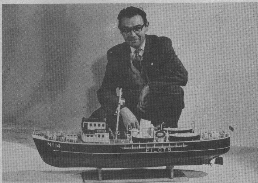
Tom Shortt, Ireland, made twin-screw Meccano gears. Two MM motors for actuation purposes. Hull length is 46 inches.
