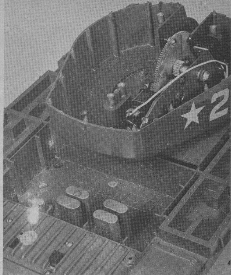
This view shows special cocking motor metal mount and micro-switch, to right of big gear, which shuts off motor when gun ready to fire. To rear of turret are four motor-control relays, switches and an antenna pin-jack on rear decking.
