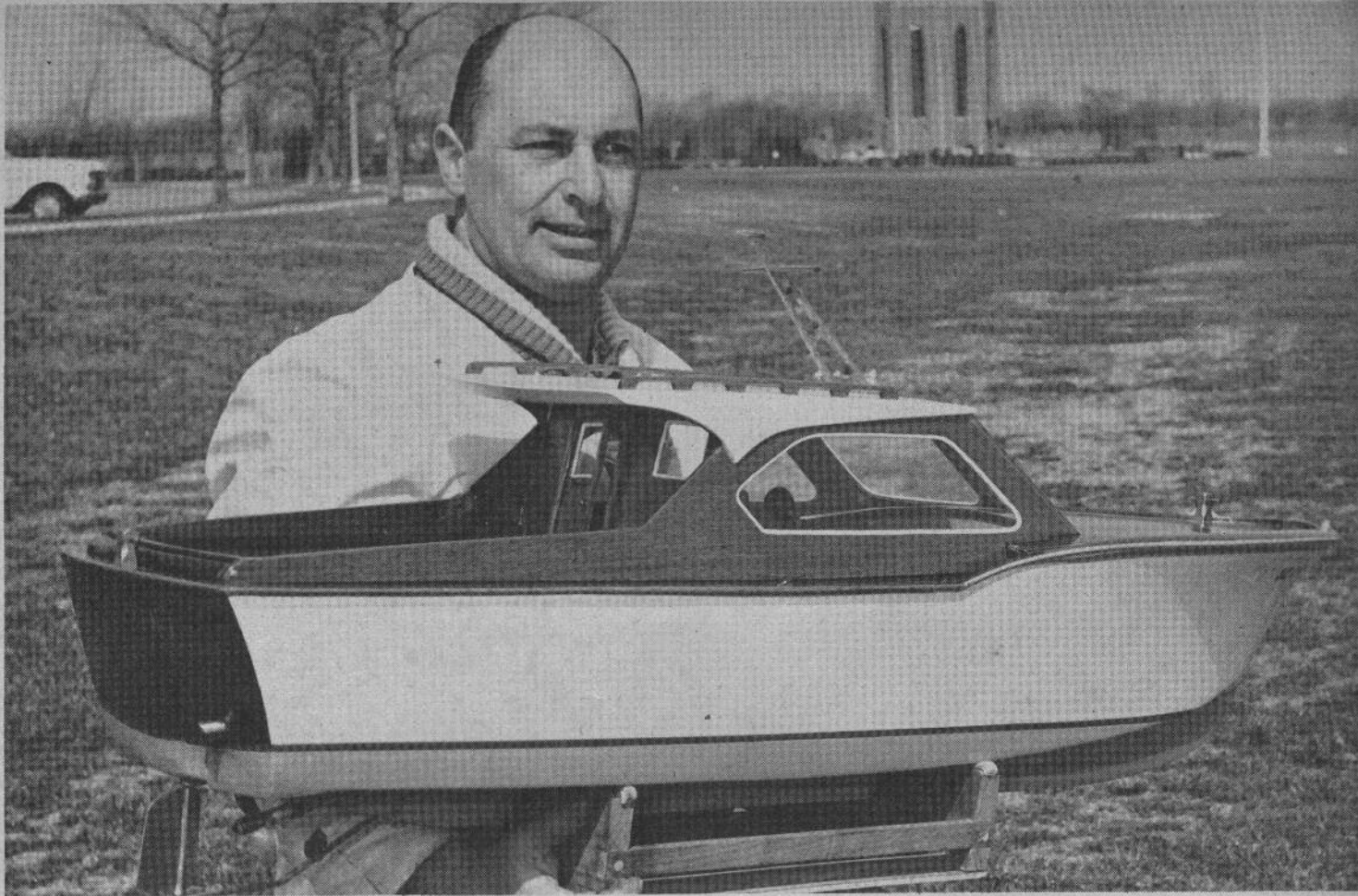
hull with substantial fiberglassing for strength. Pull-starting works well with the inboard engine and good muffler keeps interior immaculate.
