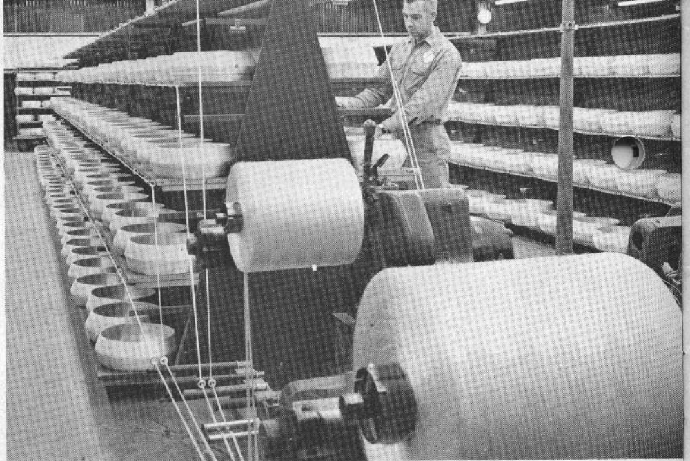
Reminiscent of a textile mill, this shot actually shows a roving machine at work.
