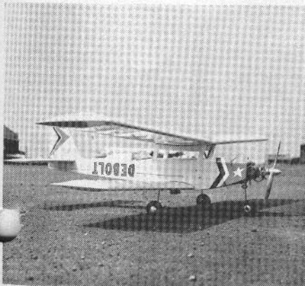
DeBolt's new biplane handles like a low-wing: 57 in., 1050 area, Super T .46.
