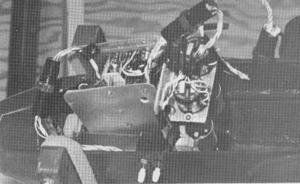
Superhet front end linked with servo amplifiers for proportional system, using feedback circuitry. Low-battery-drain setup shown in Grant Munsey's Bergfalke.
