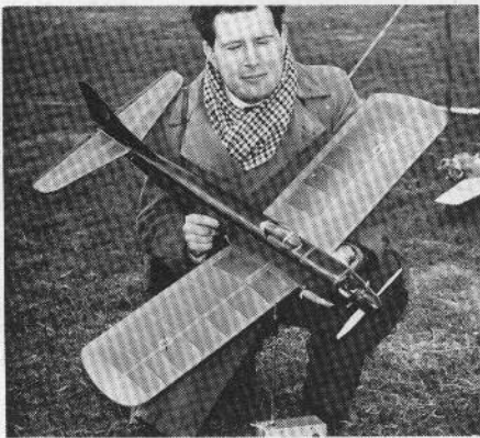
Clipped wing pylon special by C. Ralph used the RCS "Gallop Ghost" system.
