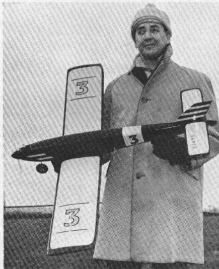
Frank Van Den Bergh's racer used all-sheet wing, one-piece frame! Cox .15.
