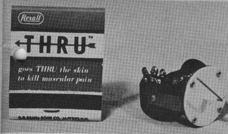
The latest Adam's actuator, a refinement of 11 years of work. Matchbox cover suggests the small size of magnetic actuator.
