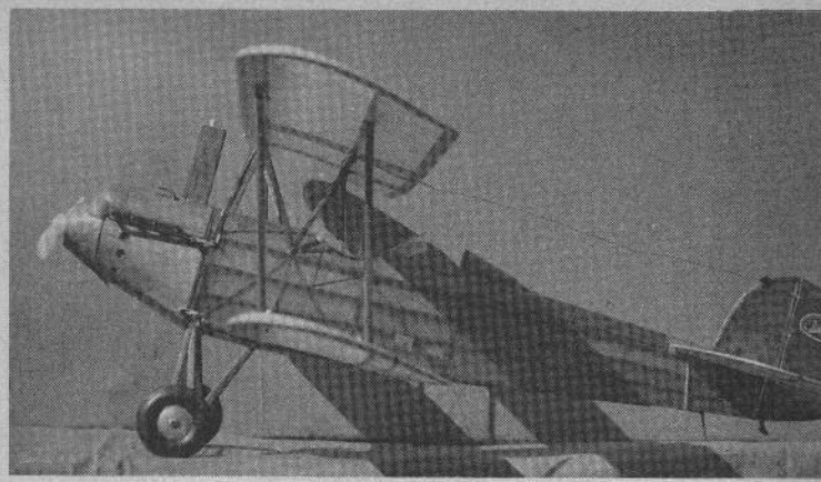
Headed "west" here, but from a slightly lower eye-level. Holes near nose mount dummy cylinders of radial engine.
