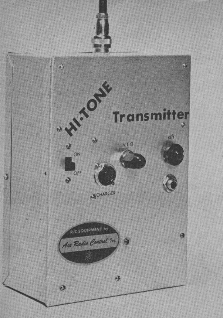
Using the PC Board on opposite page this typical transmitter was assembled. Provides for pulse-box plug, charger plug.
