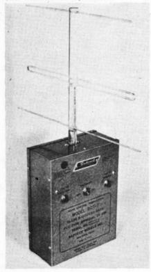
tips. The two units are very light, thin bakelite plates carrying the antennas, a bakelite plates carrying the antennas, a diode, condenser and pair of RF chokes. Receiver chassis is enclosed by a light
