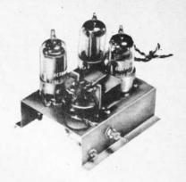
3V4 oscillator screen grid resistor has been dropped to 47K ohms. Berkeley furnishes a shorter antenna than was used with the original, since field strength tests show it to be just about as effective. Because the circuits are virtually unchanged from those in the issues mentioned, we are not printing them
