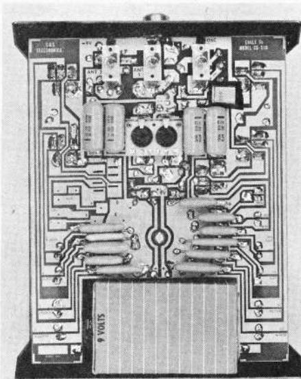
vent close range overloading. Solid state circuitry is employed throughout, including six transistors in the IF stages. The receiver cannot drift or vibrate out of alignment due to the fact that the usual adjustable transformers are replaced by the newer Cle vite Transfilters. The only tuning required was to peak the antenna circuit for maximum sensitivity with the "Eagle" transmitter.
