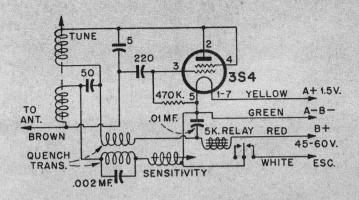
■ This single hard-tuber utilizes a form of sensitivity control not often seen in receivers made in this country, but popular in England. As you will note from the circuit, sensitivity is adjusted by means of a slug-tuned coil, and the frequency control is also of this type.
