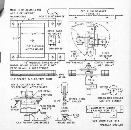
HOLES FOR MOTOR MOUNT BOARD SCREWS
