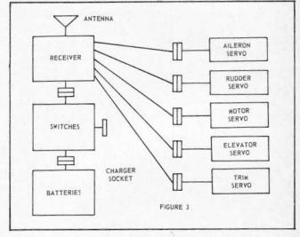
The most general type of multichannel reed system cabling is shown in this figure. This diagram relates directly to the wiring diagram on Figure 1.
