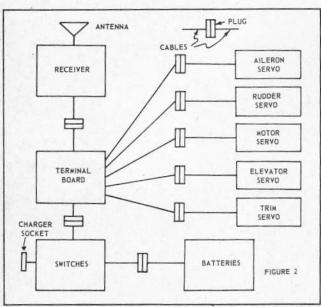
This method of multichannel reed system cabling may be used when a terminal board is included in the receiver. In this case the plug and connector with the largest number of pins is eliminated and the flexibility of the installation is not diminished.
