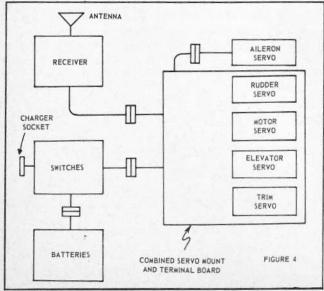
This method of multichannel reed system cabling is based on a commercially available servo mounting board which includes a printed circuit type terminal board. The number of connectors is minimized using this scheme.
