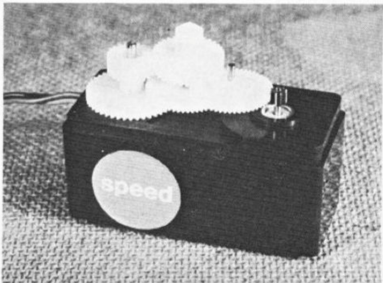
Above and below are shown the electronics and the mechanics of the "Contest" servo, a 3D 3-view at left gives layout.
