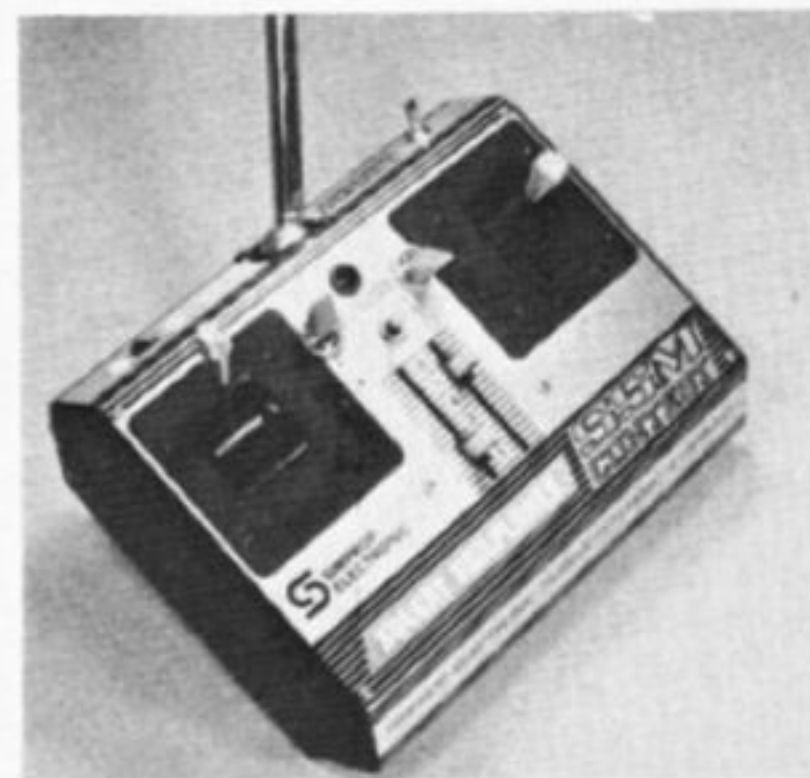
This view shows how transmitter aerial may be angled, via ball-and-socket.
