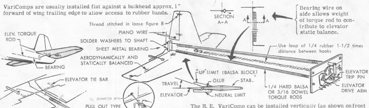
Whether eley, torque rod goes over or under elevator, and other installation details depend on the design of the airplane and references of the modeler. 2 alternate setups are shown above.
