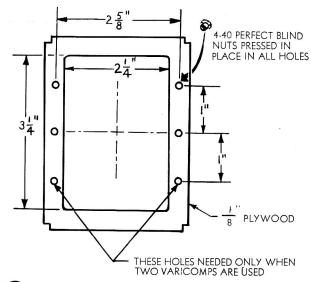
2 Install linkage support with 4-40 screws and lockwashers.
