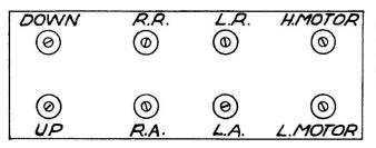
In the rear of the transmitter at the top are 8 controls accessible through holes in the back cover which permit the audio tones to be tuned exactly to the reeds in the receiver. They are arranged for maximum convenience if the receiver is connected in accordance with the instructions packed with it and are shown here. If some other arrangement of connecting the reeds is used, the following chart identifies the frequency:
