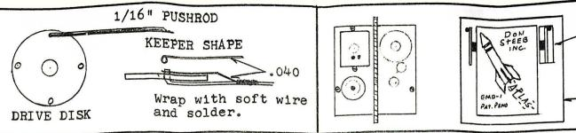
Use at least .040 piano wire keepers. Be sure linkage is free. Other methods of operating surfaces may be used. This is most trouble free. Vertical tray mounting(most crash proof). Mark all screw points on bottom of servo and drill relief holes in tray. Use # 2-56 nuts & bolts to mount.
