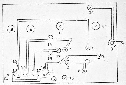
Your Ace PC2 will be easy to hook up if a few simple proceedures are followed. All you'll need in the way of tools are a small soldering iron such as Ungar 25 or  $37\frac{1}{2}$  watt, and a wire cutters. We strongly recommend the use of Ersin solder, which is furnished.
