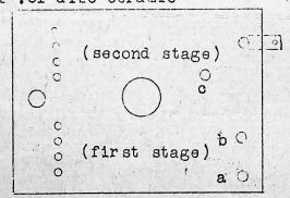
Conventional Lorenz base as it appears from underside. Eyelet c is new and must be added to present base.
