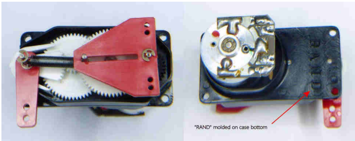
later HR-2 with "RAND" name on base and 3rd generation printed circuit filter
