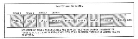
and the repetition rate of these tones. There are only two discriminators in this receiver. The outputs of the discriminators drive servos as before, but in this case, the outputs also drive rate and symmetry detectors whose outputs are D.C. voltages that vary with stick position. These voltages are fed to the other servos which operate in the same manner as the servos driven by the discriminator.
